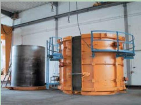
Exact amounts of the materials are pre-mixed, with the raw material quantities, mixing sequence and material feeds controlled by a computer. Then, the mixed material is loaded into vertical molds where vibratory compaction is used to ensure a dense, void-free composite structure.
